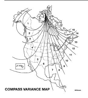
To set the variance: Turn the ignition ON and set the display to "Compass/Temperature." Press the C/T button for approximately 5 seconds. The last variance zone number will be displayed. Press and hold the STEP button for 1 second to select the new variance zone and press the RESET button to resume normal operation.
