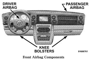
This vehicle has airbags for both the driver and right front passenger as a supplement to the seat belt restraint systems. The driver's front airbag is mounted in the steering wheel. The passenger side airbag is mounted in the instrument panel, above the glove compartment. The words SRS/AIRBAG are embossed on the airbag covers.
