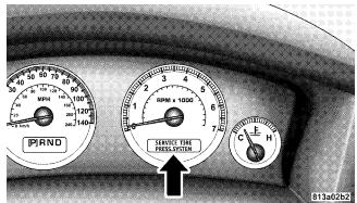
The electronic vehicle information center (EVIC) located in the instrument cluster, when the appropriate conditions exist, will display the following messages and symbols. Some of the messages are accompanied by a chime.
