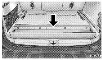
**Cargo Load Floor** 4. Pull up on loop(s) and twist 90 degrees, so they are perpendicular (straight up) to the slotted hole in tray. 5. Push loop(s) back down, so they are parallel to the top of the tray.
