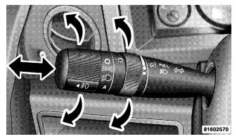
Headlight Switch Automatic Headlight System — If Equipped Turn the end of the multi-function control lever to the third detent to activate the automatic headlight system.
